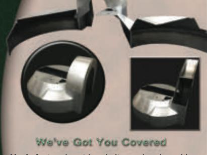
May's featured part is a belt guard and machine cover. It is also a 27pc jigsaw puzzle. Once the pieces are laser cut, they travel to the forming department to be bent, rolled, and tweaked into shape. From there the parts go to the welding department where the real fun starts. As you can see from the photos there are four weldment sections that are connected with hinges. Our skilled welder carefully aligns all of the pieces to create the articulating masterpiece shown here.
