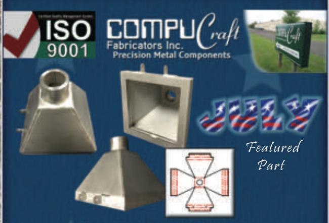
For July we are featuring the funnel assembly shown here. The first step in the fabrication process is to laser cut the flat pattern shown above (see inset). The flat pattern is then formed along the bend lines, represented in red on the inset diagram. Once formed into the funnel shape, the intersections are welded, in addition to welding on the bezel, hinge tabs, and output tube. Finally the part is passivated to remove weld burn prior to inspection and shipping.
