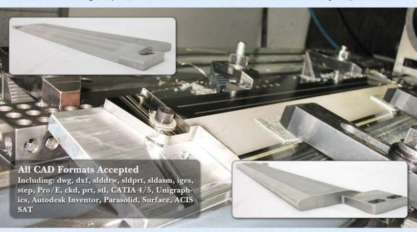
CAM, or Computer-Aided Manufacturing, is the use of computer software to control machinery in the manufacturing of workpieces. This month we are featuring a part that was machined directly from a 3D CAD file provided by our customer. By leveraging the the ability of our skilled machinists with advanced computer software we are able to produce more complex parts in less time than with traditional machining practices.
