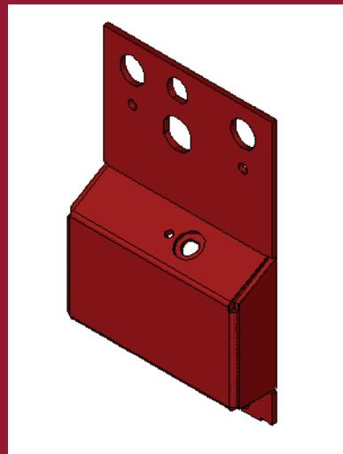
*Top Left:* Flat pattern developed using KeyCreator CAD software. *Top Right:* Formed part with hardware, prior to welding. *Far Left:* Finished part. Supplied to our customer with paint and silkscreen per their specifications. *Left:* Isometric CAD view of part.
